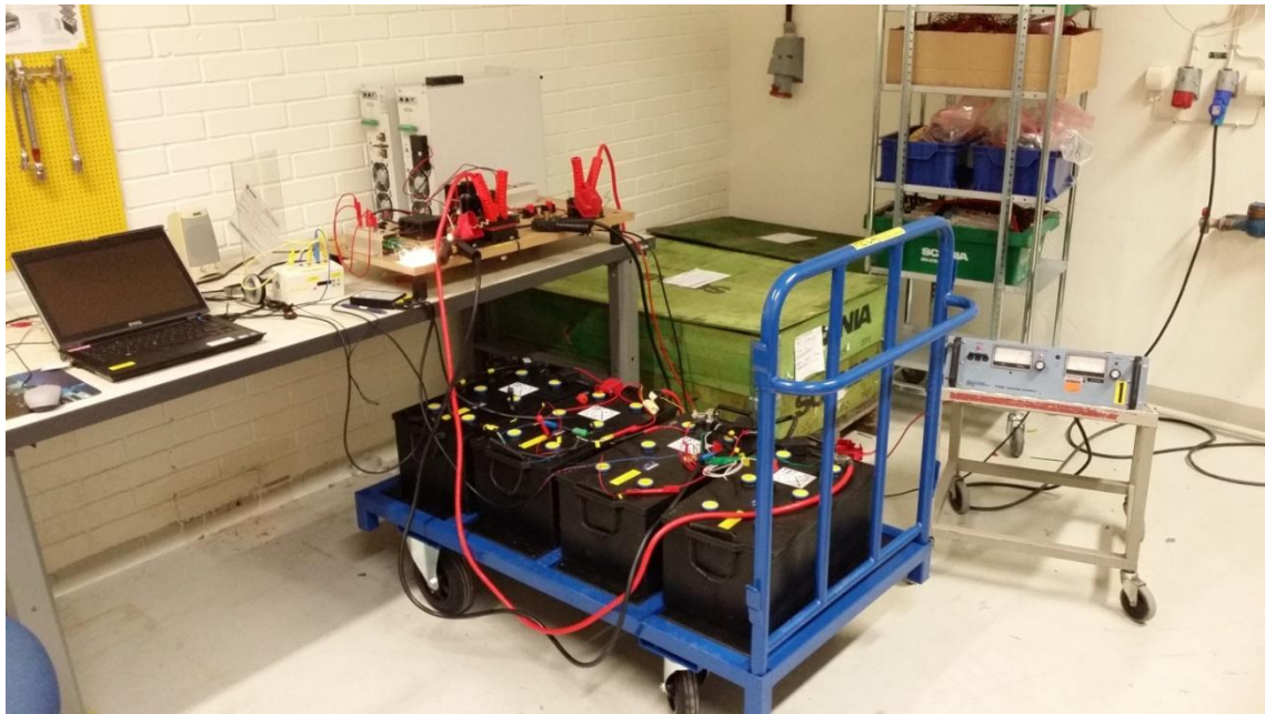
Figure 15: The entire test bench, with batteries, power supply, loads and computer to log the data.
