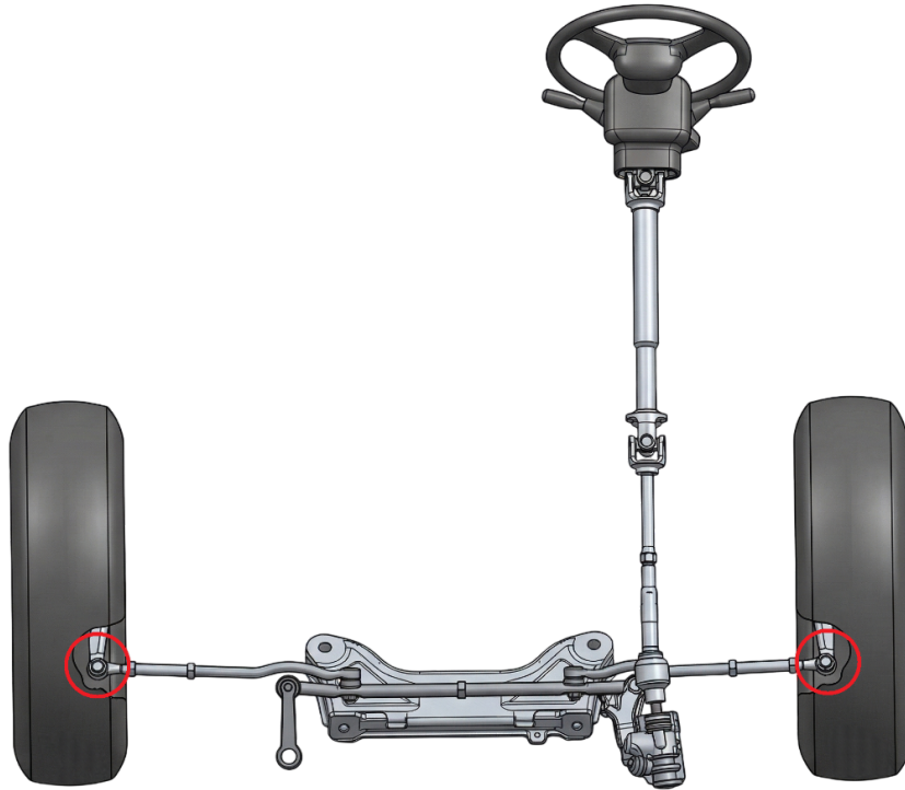
Figure 9. Steering angle sensors are placed in the steering knuckles, marked by the red rings. 3
