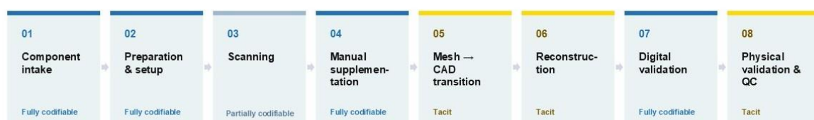
Figure 5.2. Eight-stage reverse-engineering workflow, with codifiability level per stage. Fully codifiable stages: 1, 2, 4, 7. Partially codifiable stages: 3. Tacit stages: 5, 6, 8.
