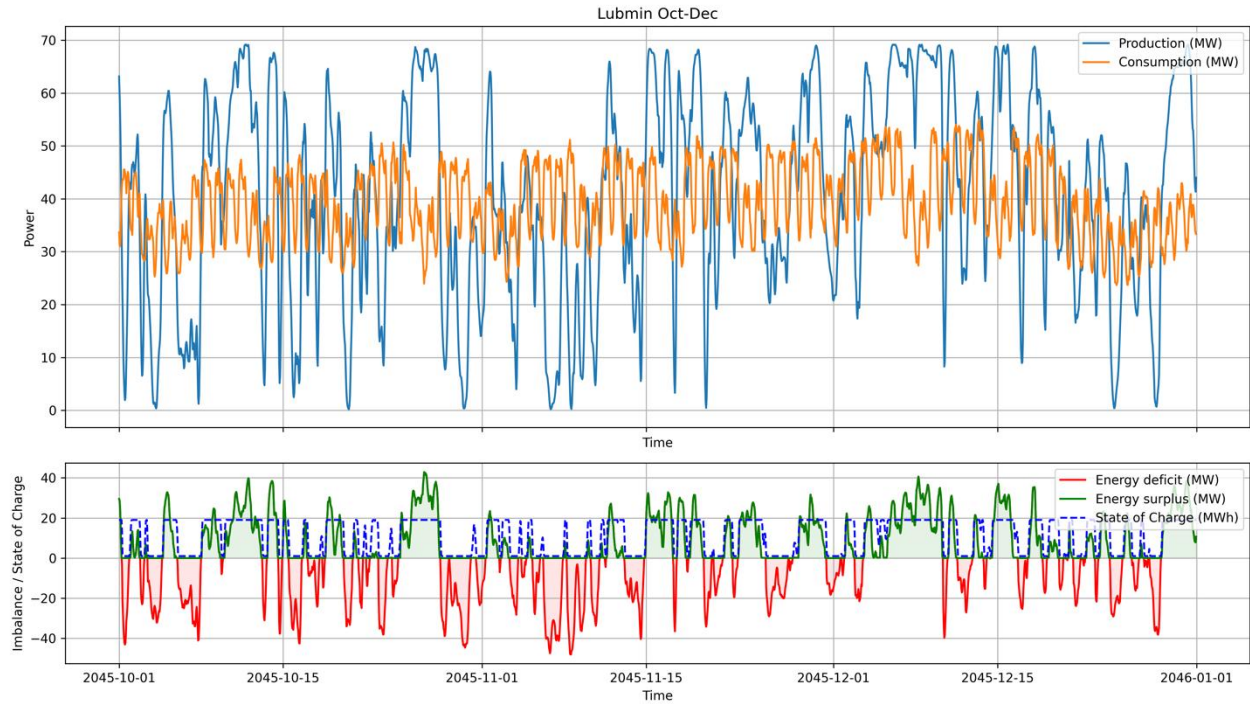
Figure 14. The upper graph shows the difference in production vs consumption. The lower graph shows energy balance and battery operation at the Lubmin site for the fourth quarter of 2025.
